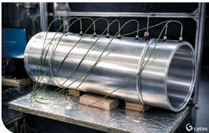
Figure 1. Testing setup used to assess equipment performance under hydrogen-methane operating conditions.
