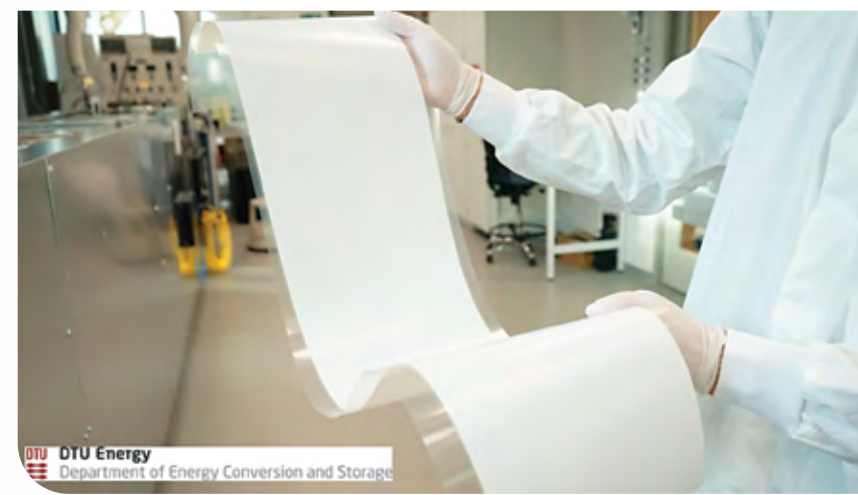
Green tape of electrolyte layer for a solid oxide cell (SOC), made using the tape caster at DTU Energy to the left. The electrolyte layer is on top of a plastic band, that is later removed. All the layers of the SOC are put together and sintered giving stiff cell at the end
