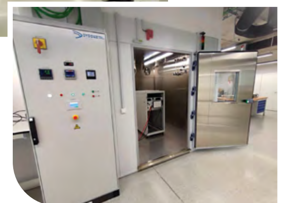
100 kW 2.5m x 2.5 x 2.0m environmental test station for hydrogen technologies -40 to 70°C automated operation
