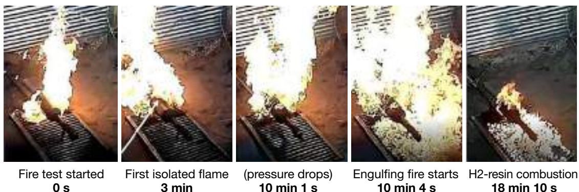
Figure 1. Self-venting NWP=700 bar tank prototype in localised and engulfing fire portions of HRR/A=1 \text{ MW/m}^2 intensity 28 .
