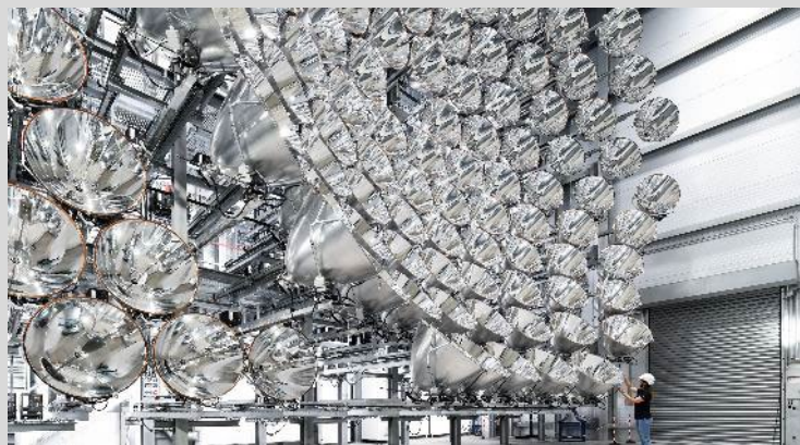
DLR Synlight: World's largest solar simulator
