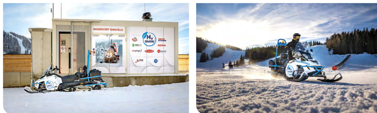
Figure 5: Hydrogen filling station for HySnow (left) and fuel cell snowmobile (right)
