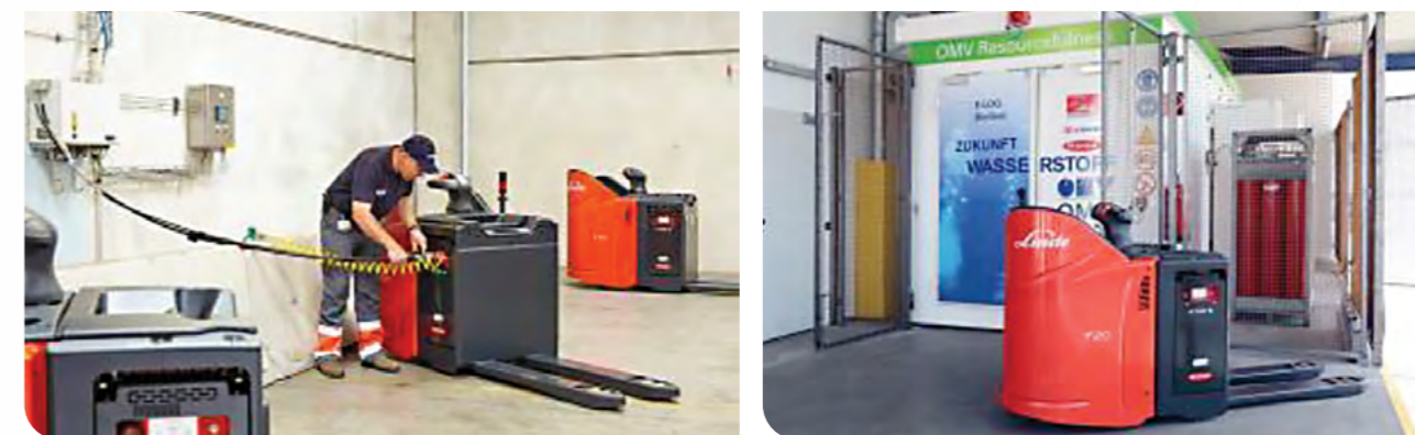
Figure 3: Project E-LOG BioFleet I & II with indoor refuelling infrastructure (left) and hydrogen production on-site (right)
