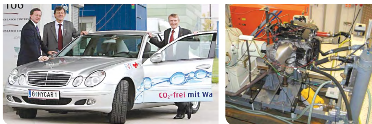
Figure 2: Project HyCar, adapted Mercedes Benz E200 (left); engine adaptations on test bench (right).
