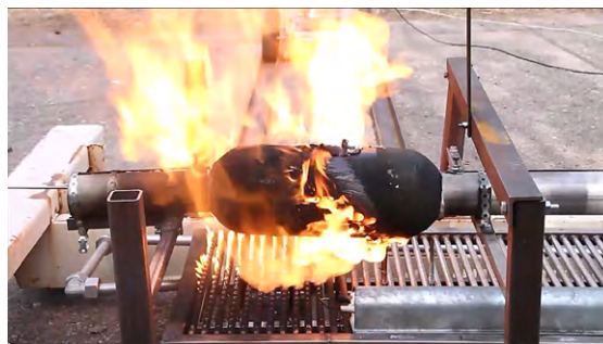
Burner fuel supply stopped, resin is still burning
