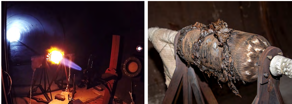
Figure 3. Self-venting tank prototype under extreme impinging jet fire of highest ever intensity of HRR/A=19.5 \text{ MW/m}^2 from a 700-bar storage tank: left – during fire test, right – aftermath of the prototype composite of tank test 30 .
